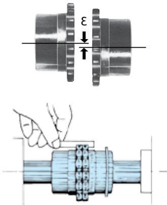
In the case where sprocket r/min is 1/3 or more of the maximum r/min, the allowable angular and parallel misalignments are  $0.5^\circ$  and 1% of the chain pitch
