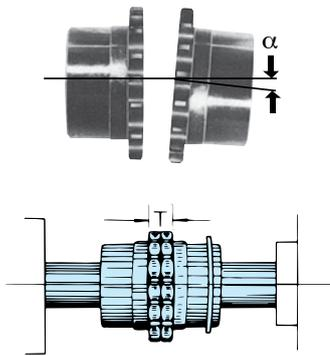
Place a straight edge at the bottom of corresponding teeth of the two sprockets and adjust so that parallel misalignment is minimized. Allowable parallel misalignment ( $\epsilon$ ) is 2% of the chain pitch.
