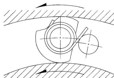
Figure 3: Inner and outerrace locked and turning
