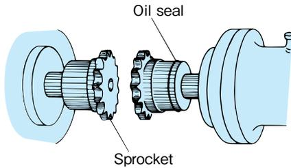
2. Bring the sprocket faces close together and correct the angular and parallel misalignment.
